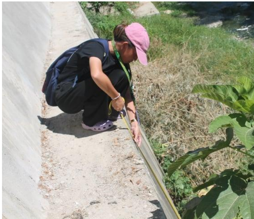
Fig 2.2 Measurement of new riprap is 200-250 cm
